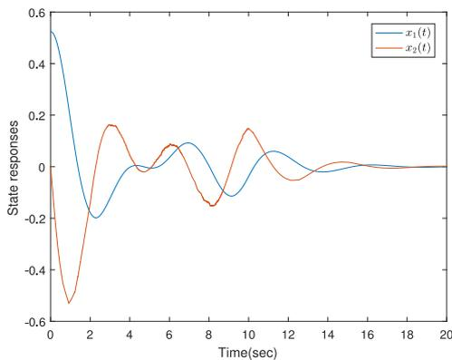
Fig. 8. State responses of the system with deception attacks by using standard controller in (33).
